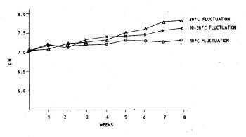
Figure 2. Effect of temperature on pH profile
