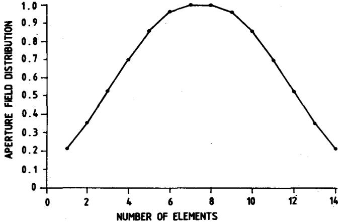
Figure 2 (b). Aperture voltage distribution in the elevation plane.
