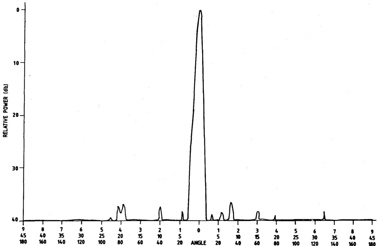
Figure 4 (a). Radiation pattern of the planar array in azimuth plane
