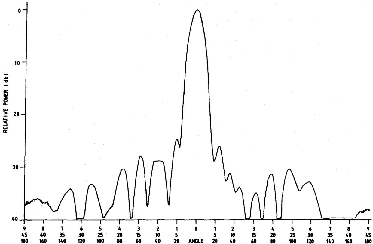
Figure 4 (b). Radiation pattern of the planar array in elevation plane
