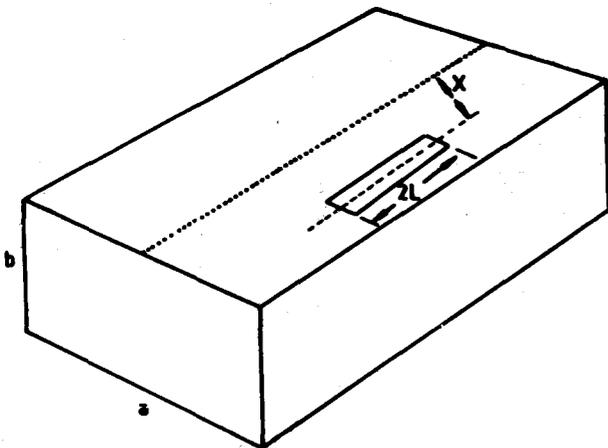
Figure 1. Slot cut on top of rectangular waveguide showing basic element used in the planar array.
