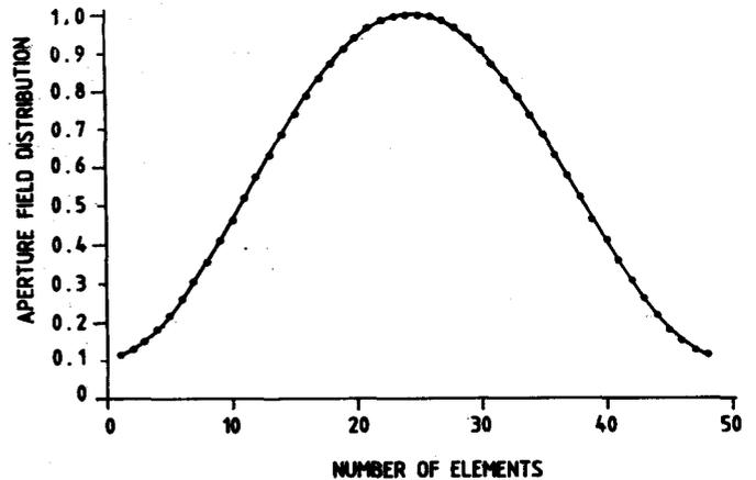
Figure 2 (a). Aperture voltage distribution in the azimuth plane.
