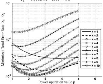
Figure 10. Minimized total error rate  $Q_m + Q_f vs P$  for different k, SNR = -5 dB, M = 10, N = 50.
