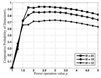
Figure 8. Maximized cooperative probability of detection  $Q_d vs P$  for different M, SNR = -5 dB,  $Q_f = 0.0001$ , N = 50.
