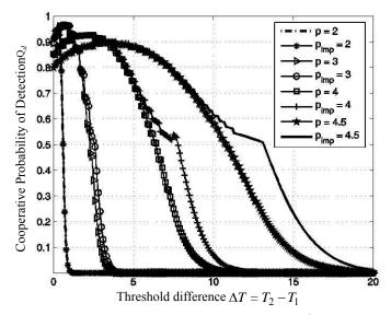
Figure 11. Cooperative probability of detection  $Q_d$  vs  $\Delta T$ for different p for imperfect reporting channel with  $P_{\rho} = 10^{-3}$ , SNR = -5 dB.
