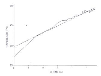
Figure 3. Graphical PC output of temperature with time on logarithmic scale and straight line curve fitting for glycerol.
