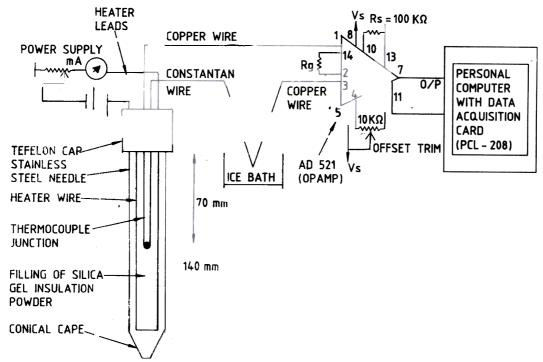
Figure 1. Electronic diagram of thermal conductivity measurement system
