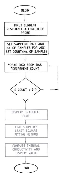
Figure 2. Flow chart for PC-based thermal conductivity measurement system.
