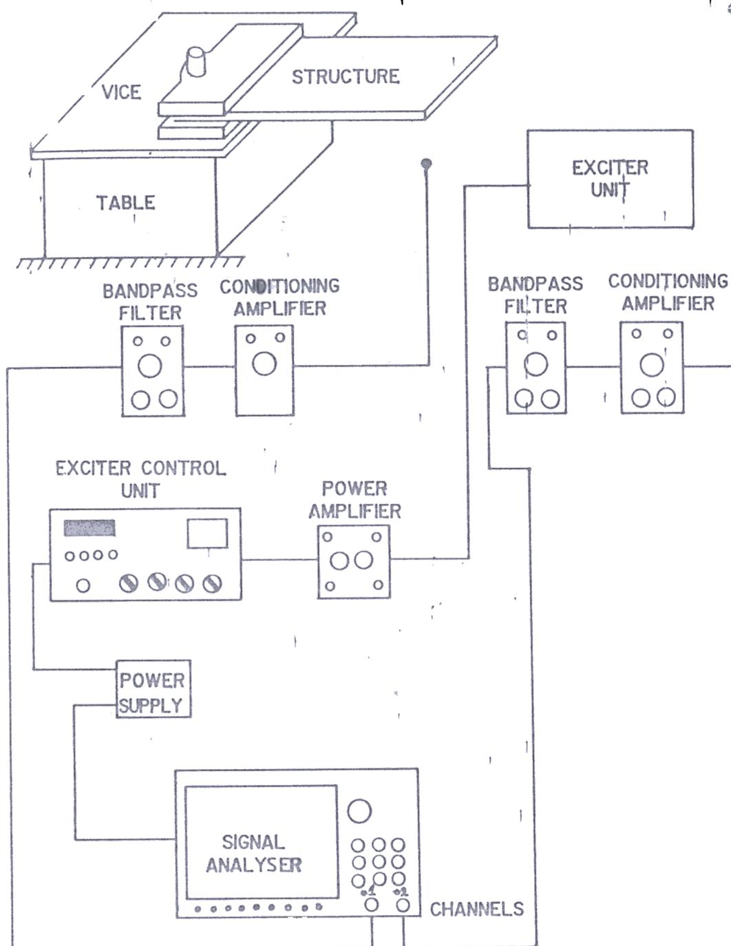
Figure 1. General schematic experimental setup
