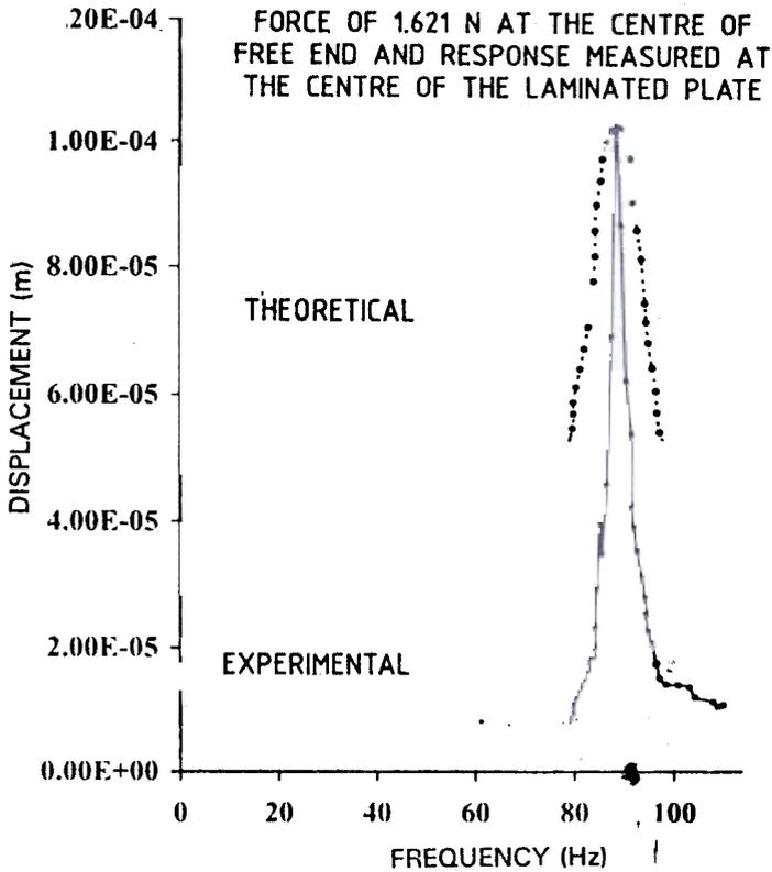
Figure 3. Frequency response of laminated cantilever 11-layered plate.
