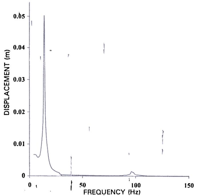
Figure 4. Frequency response of laminated cantilever 11-layered beam.
