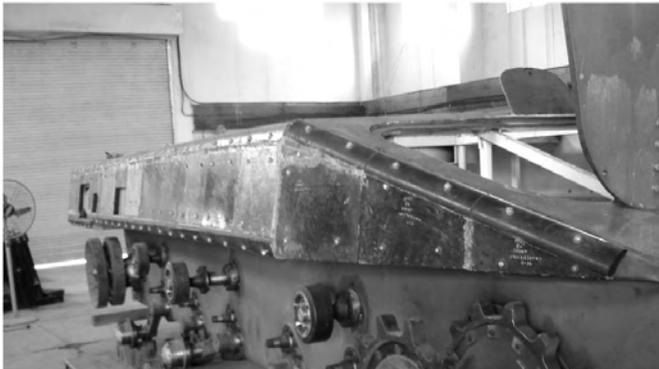
**Figure 6. Ceramic armour components fitted on the experimental infantry combat vehicle.**
