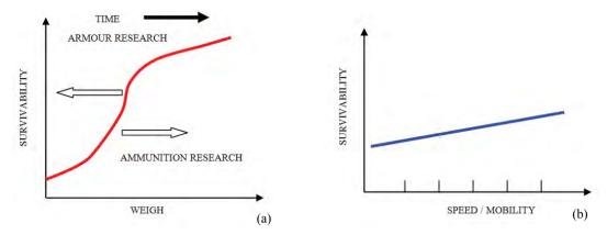
Figure 10. Survivability as a function of: (a) weight, and (b) mobility.
