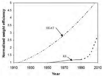
Figure 2. Improvements in armour efficiencyin tanks.
