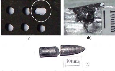
Figure 5. Photograph of: (a) perforated high hardness steel plate, (b) depth of penetration in backing *Al*-7017 alloy, and (c) fractured projectile after the impact.
