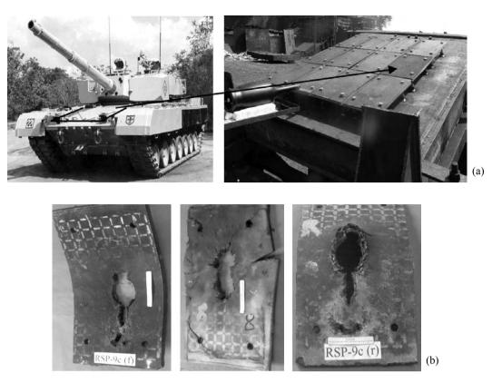
Figure 7. Ballistic evaluation of dynamic passive armour against HEAT missile: (a) test set-up, and (b) damage of the cassette material.
