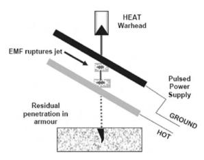
Figure 9. Principle of electromagnetic armour.
