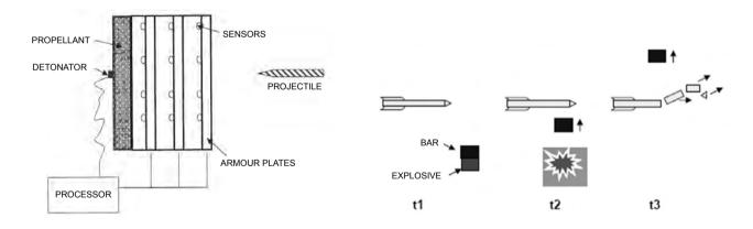
Figure 8. Schematic concept of an intelligent dynamic armour.
