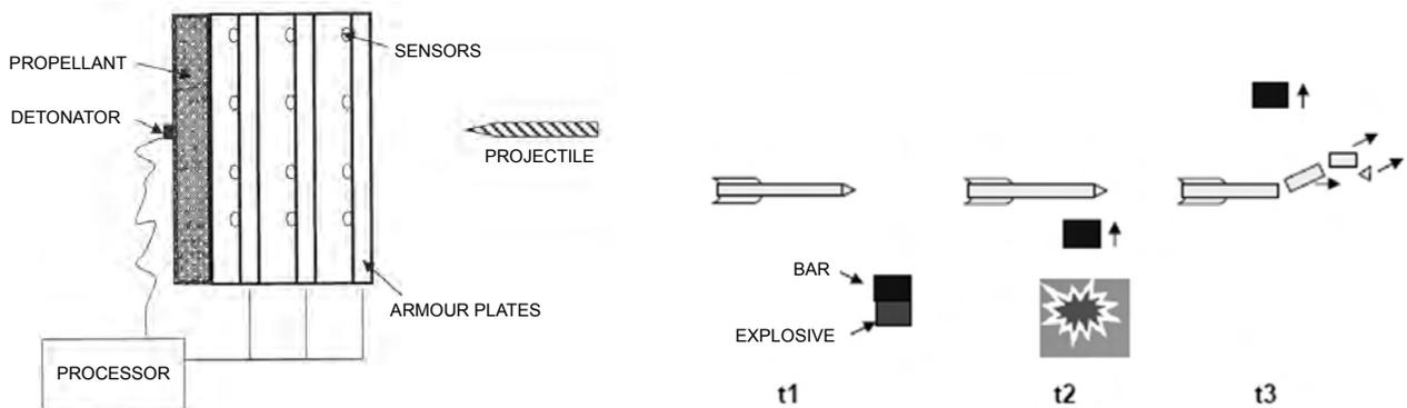
Figure 8. Schematic concept of an intelligent dynamic armour.
