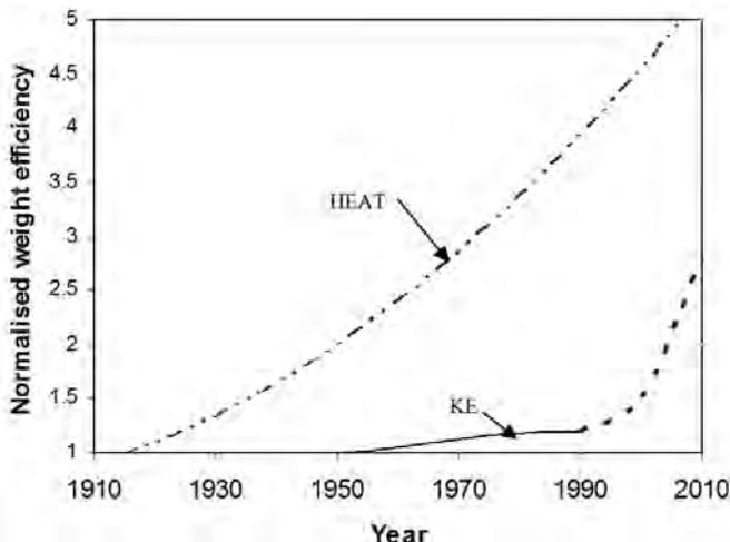
Figure 2. Improvements in armour efficiency in tanks.
