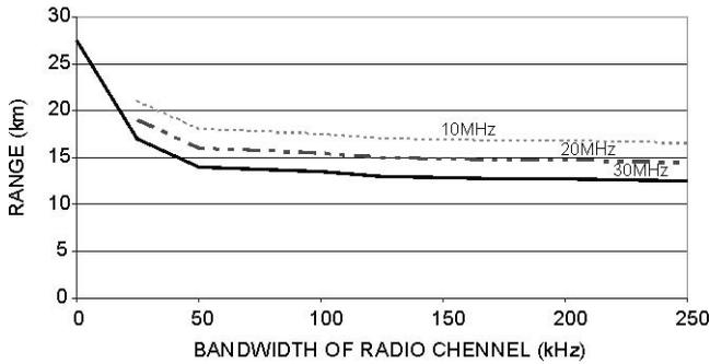
**Figure 2. Range as a function of the bandwidth of radio channel.**
