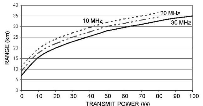
**Figure 1. Range of radio signal as a function of transmit power with frequency as parameter.**
