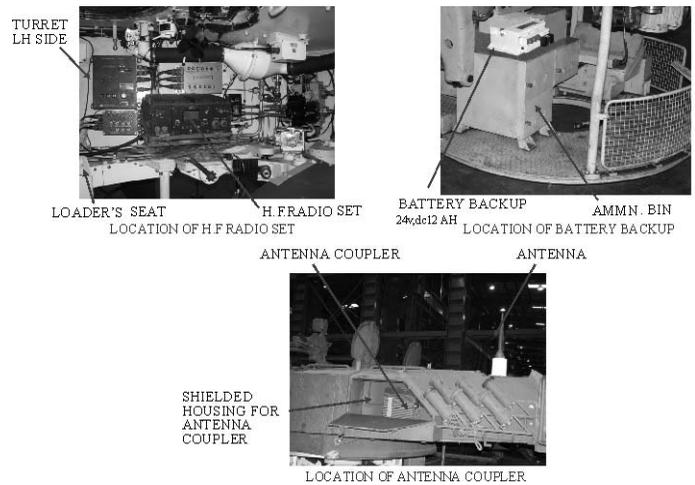
Figure 5. Communication system layout configuration-Option III
