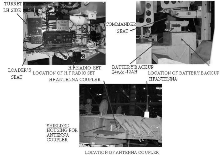
Figure 4. Communication system layout configuration-Option II.
