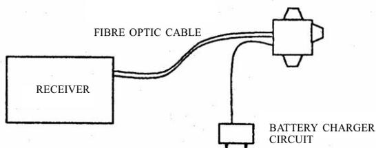
Figure 7. Test instrumentation for field monitoring.
