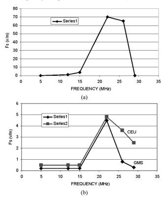
Figure 8. Measured RMS field profile of the vehicle (inside): (a) VHF radio set 1 and (b) CEU and GMS.
