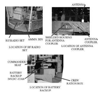
Figure 3. Communication system layout configuration-Option I.
