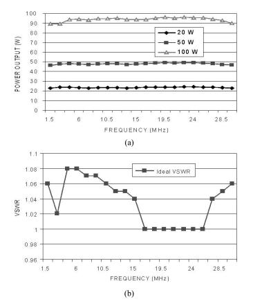
Figure 9. (a) RF power output of HF radio set and (b) ideal VSWR plots at bench.
