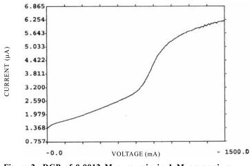
Figure 2. DCP of 0.0012 M curcumin in 1 M ammonium tartrate at  $pH 8.1 \pm 0.1$ .
