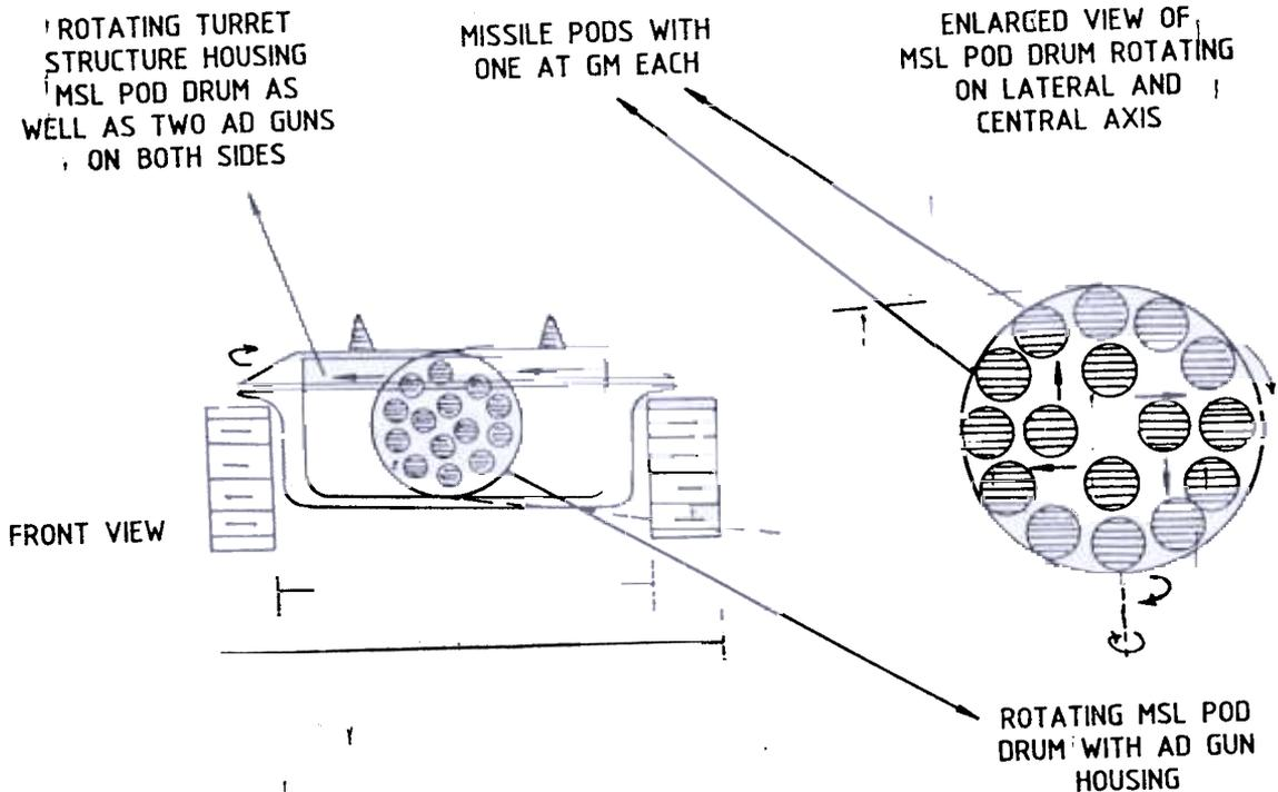
Figure 2. Front view of hybrid antitank & air defence armoured vehicle
