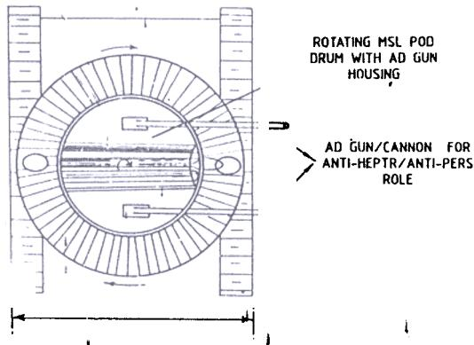
Figure 3. Top view of antitank & air defence armoured vehicle
