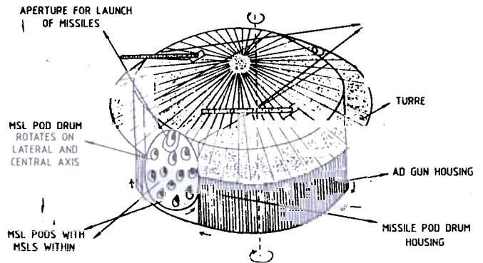
Figure 4. Tank turret with rotating MSL pod drum under it
