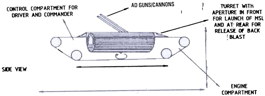
Figure 1. Design of hybrid antitank & air defence armoured vehicle
