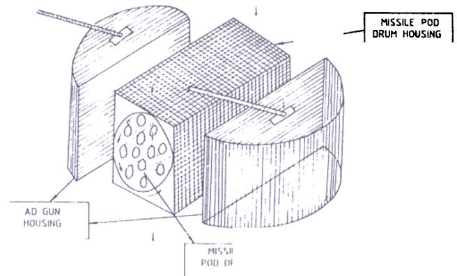
Figure 5. Rotating MSL pod drum and air defence gun housing (detached view).
