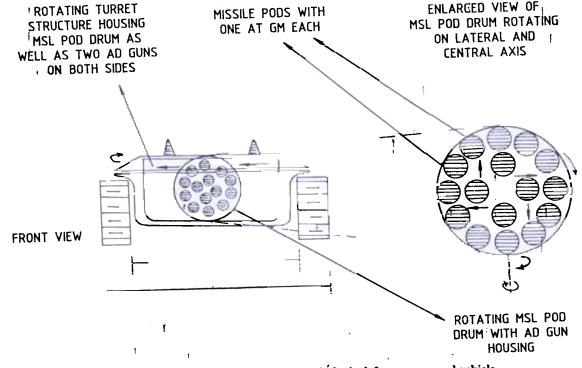
Figure 2. Front view of hybrid antitank & air defence armoured vehicle
