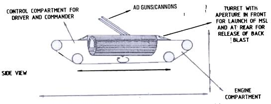
Figure 1. Design of hybrid antitank & air defence armoured vehicle
