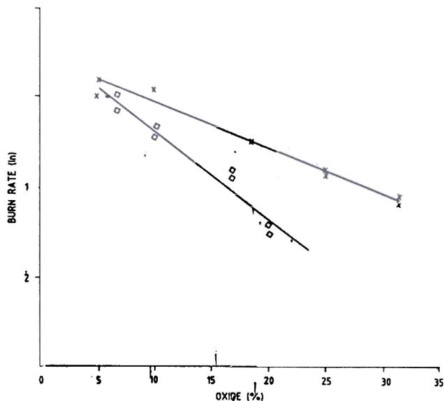
Figure 3. Plot of (burn rate) vs oxide percentage for  $Ti/KClO_4/C_2Cl_6$ /oxide smoke composition  $\square TiO_2$  and  $\times ZnO$ .
