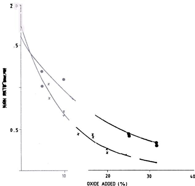
Figure 2. Effect of addition of •  $ZnO/C_2Cl_6$  (3:1 mol ratio) and  $\times TiO_2/C_2Cl_6$  (3:2 mol ratio) to the smoke composition  $Ti/KClO_4/C_2Cl_6$  (17.4 : 25 : 57.6 wt per cent).
