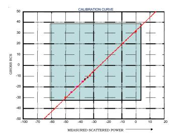
Figure 6. Multi target calibration curve at X band.
