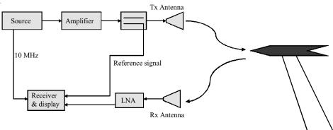
Figure 4. Basic diagram of RCS measurement.
