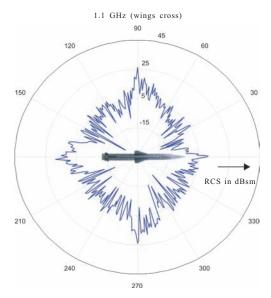
Figure 9. Predicted RCS at 1.1 GHz of actual target from 1/10<sup>th</sup> scale model measurement.
