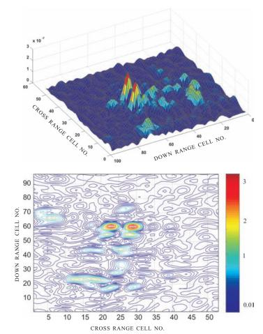
Figure 11. Two dimensional RF imaging of a complex target.
