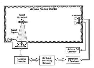
Figure 2. Anechoic chamber-far-field range.
