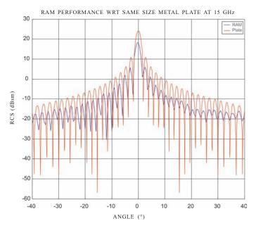
Figure 7. Measured results on 1 sqft metallic plate and RAM-coated 1 ft plate.
