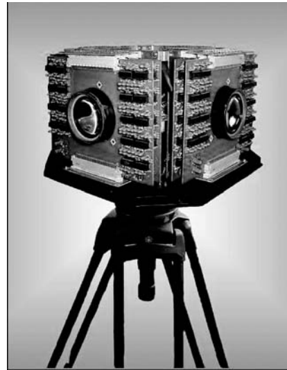
Figure 8. Precision laser warning sensor for AFVs developed at LASTEC.
