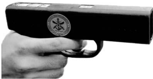
Figure 7. Hand-held short-range laser dazzler developed at LASTEC.
