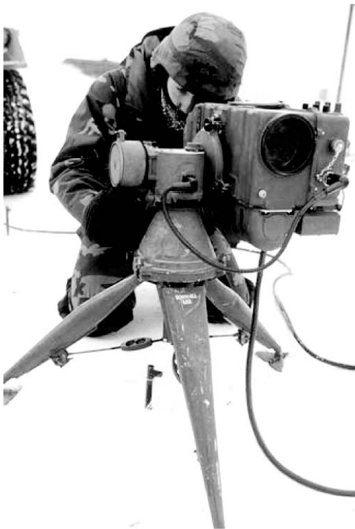
Figure 2. Portable ground-based laser designator.
