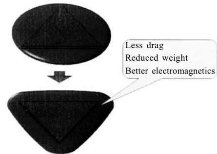
Figure 14. Optimising the non-rotating 360°-capable fixed radome.
