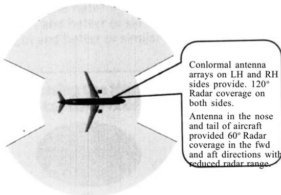
Figure 12. Conformal fuselage-mounted antenna.
