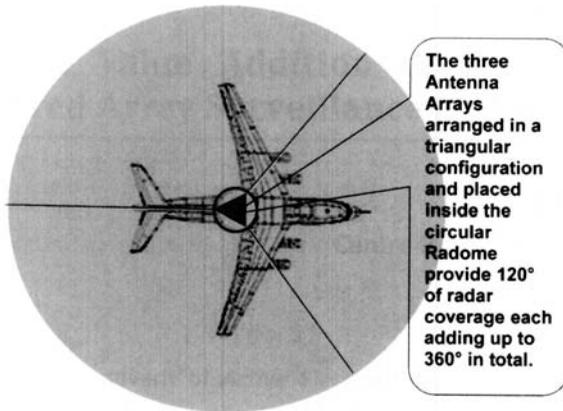
Figure 13. Triangular radome-mounted antennae.
