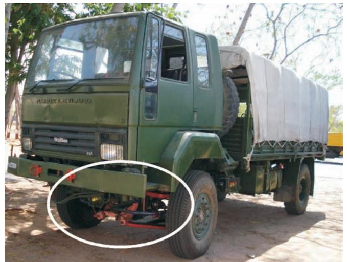
Figure 10. Independent suspension system integrated with the vehicle.
