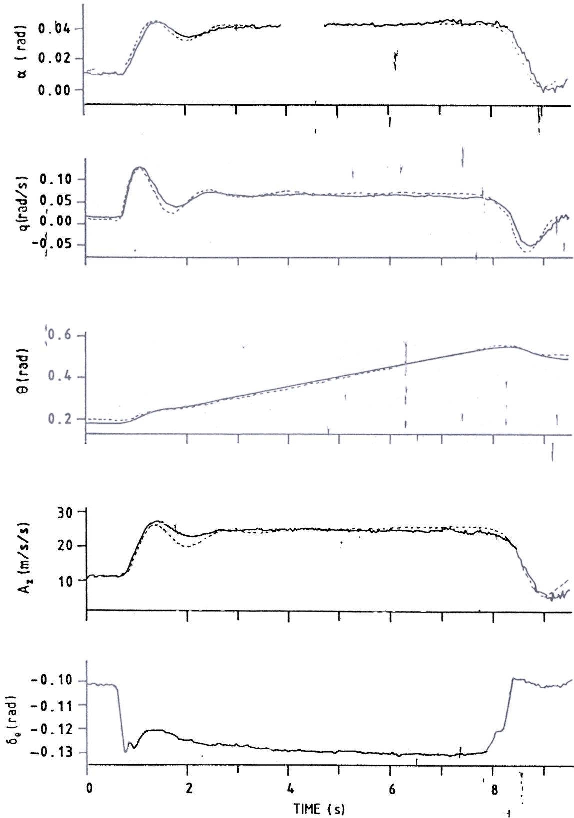
Figure 3. Time history match (parameter estimation, step input) (cross-validation, \_\_\_ FL $\hat{\Lambda}$ , ... ESTM)
