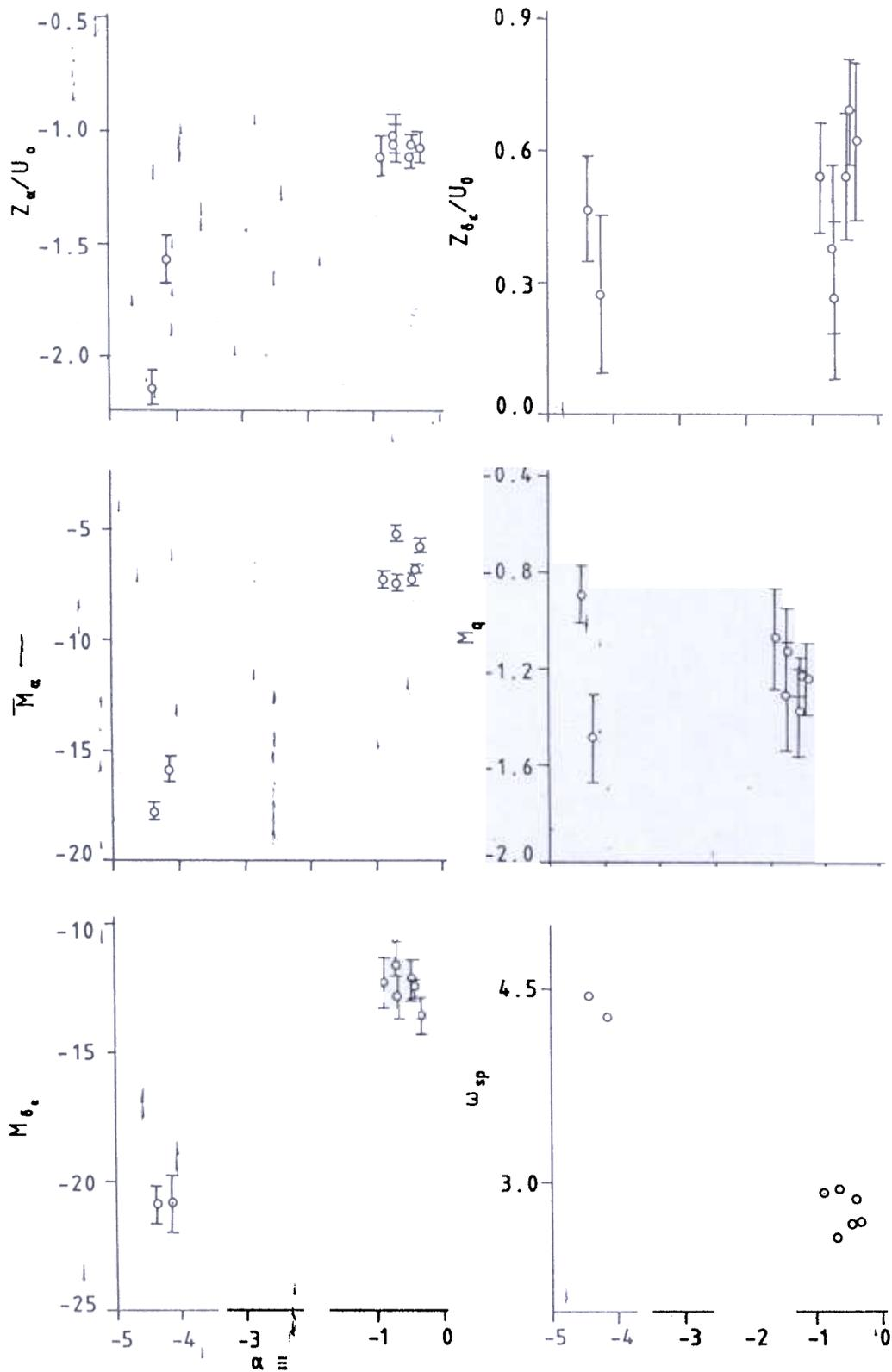
Figure 4. Variation of derivatives with angle of attack ( $\alpha$ )
