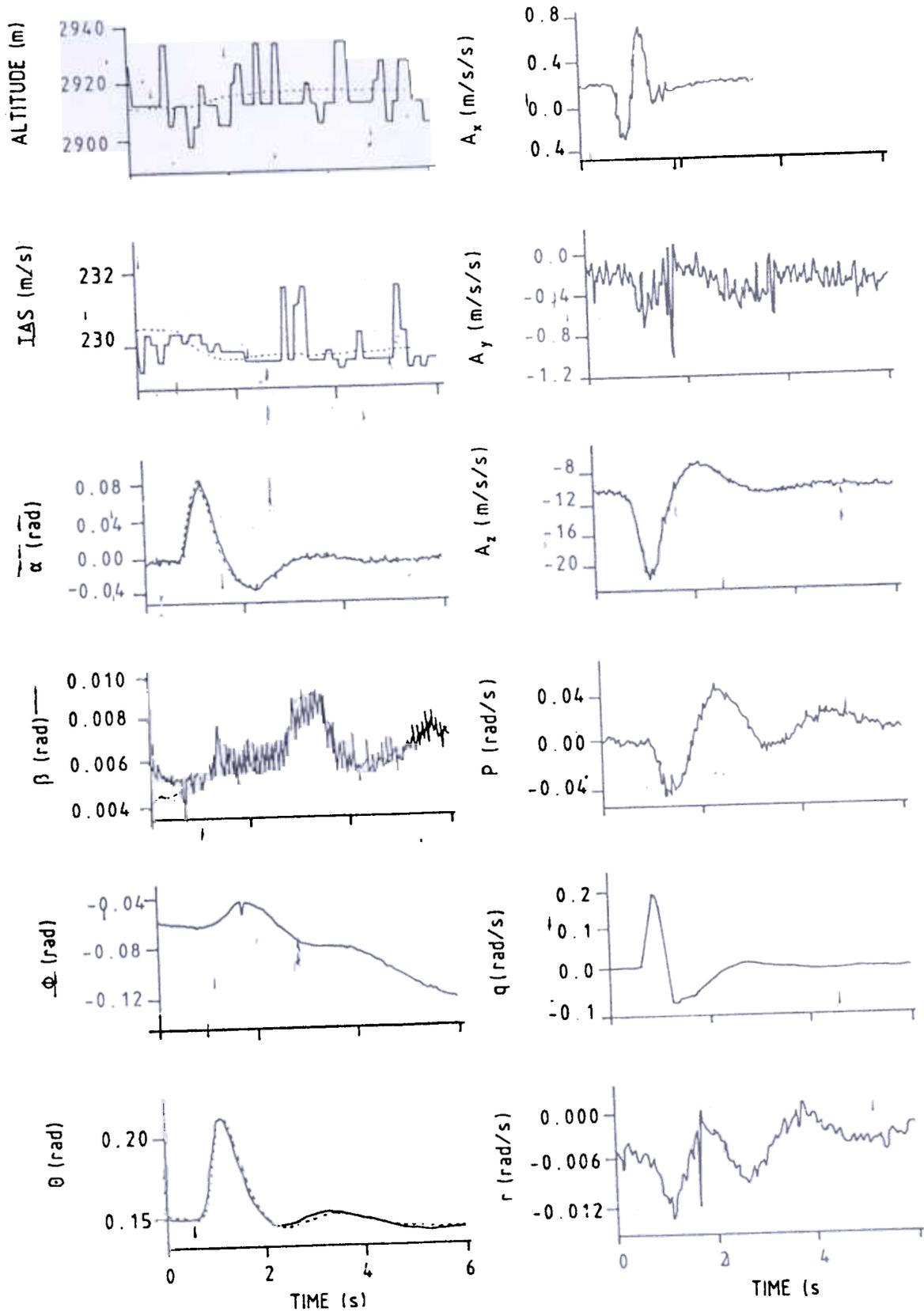
Figure 1(a). Data compatibility check (coupled model); (doublet input, \_\_ FLT, --- ESTM)
