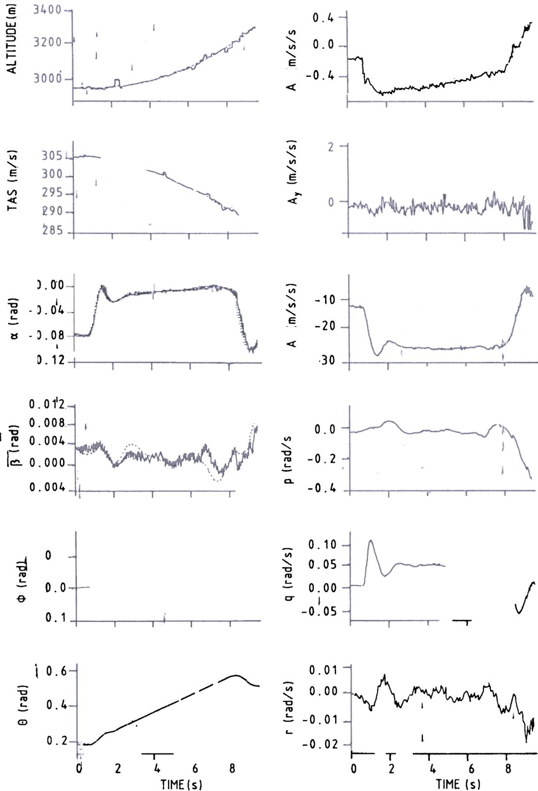
Figure 1(c). Data compatibility check (coupled model); (step input, FLT, ESTM)
