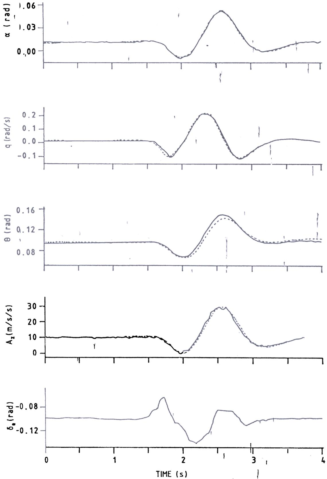
Figure 2(a). Time history match (parameter estimation, short period) (doublet input, FLT, ... ESTM)
