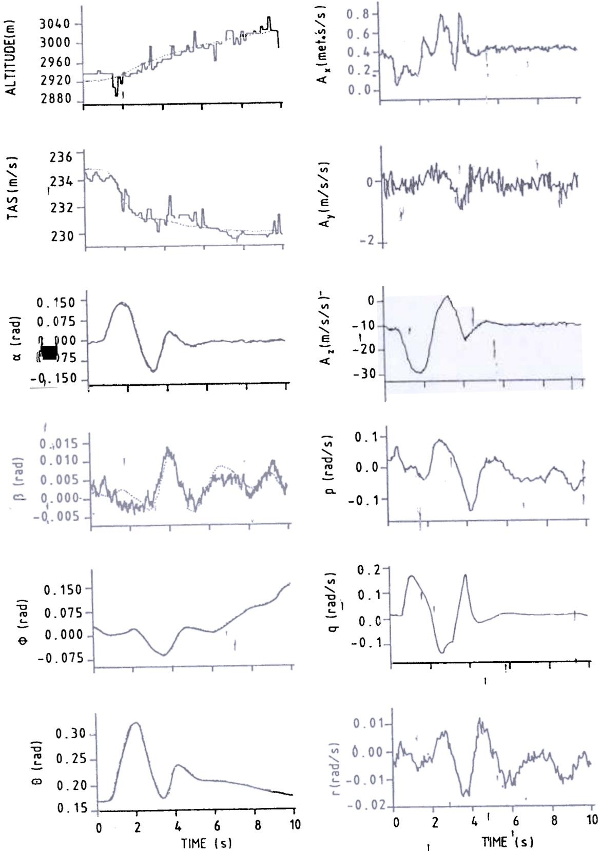
Figure 1(b). Data compatibility check (coupled model); (3211 input, \_\_\_ FLT, --- ESTM)
