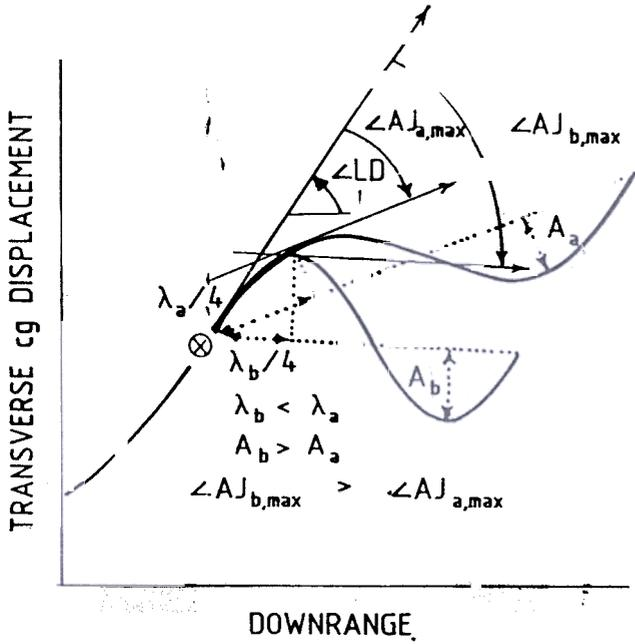
Figure 7. Depiction of variation in  $\angle AJ_{max}$  with amplitude and wavelength of the swerve curve.
