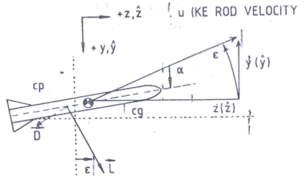
Figure 8. Illustration of the lift and drag force directions, as well as the cg velocity and the cg and cp locations.
