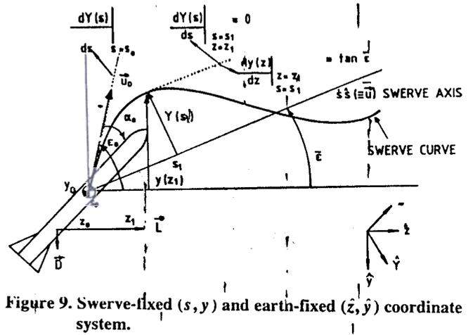
Figure 9. Swerve-fixed ( $s, y$ ) and earth-fixed ( $z, y$ ) coordinate system.
