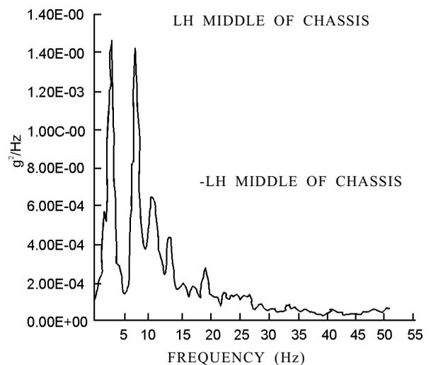
Figure 18. PSD spectra (LH middle of chassis).
