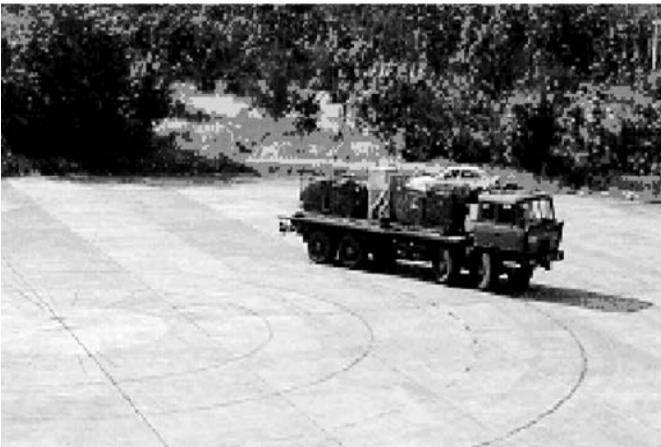
Figure 20. Safe turning speed test on steering pad.
