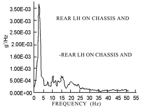
Figure 17. PSD spectra (Rear LH on chassis end).
