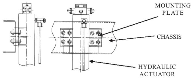
Figure 3. Hydraulic actuator as bolted to vehicle chassis.
