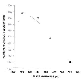
Figure 3. Variation of plugging velocity with plate hardness
