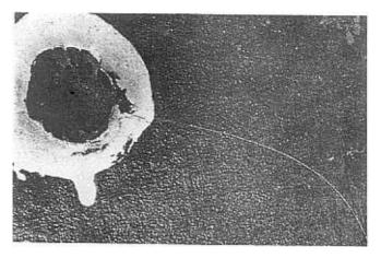
Figure 5. Deep crack formation in 20 mm thick steel armour plate at high hardness (520 HV), when impacted by 20 mm diameter steel projectile at normal.
