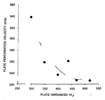
Figure 2. Variation of perforation velocity with plate hardness
