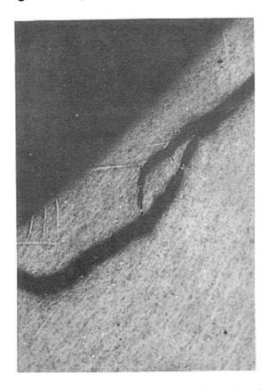
Figure 4. Formation of adiabatic shear bands near the edge of the crater in 20 mm thick steel armour plate at high hardness (520 HV), when impacted by 20 mm diameter steel projectile at normal.
