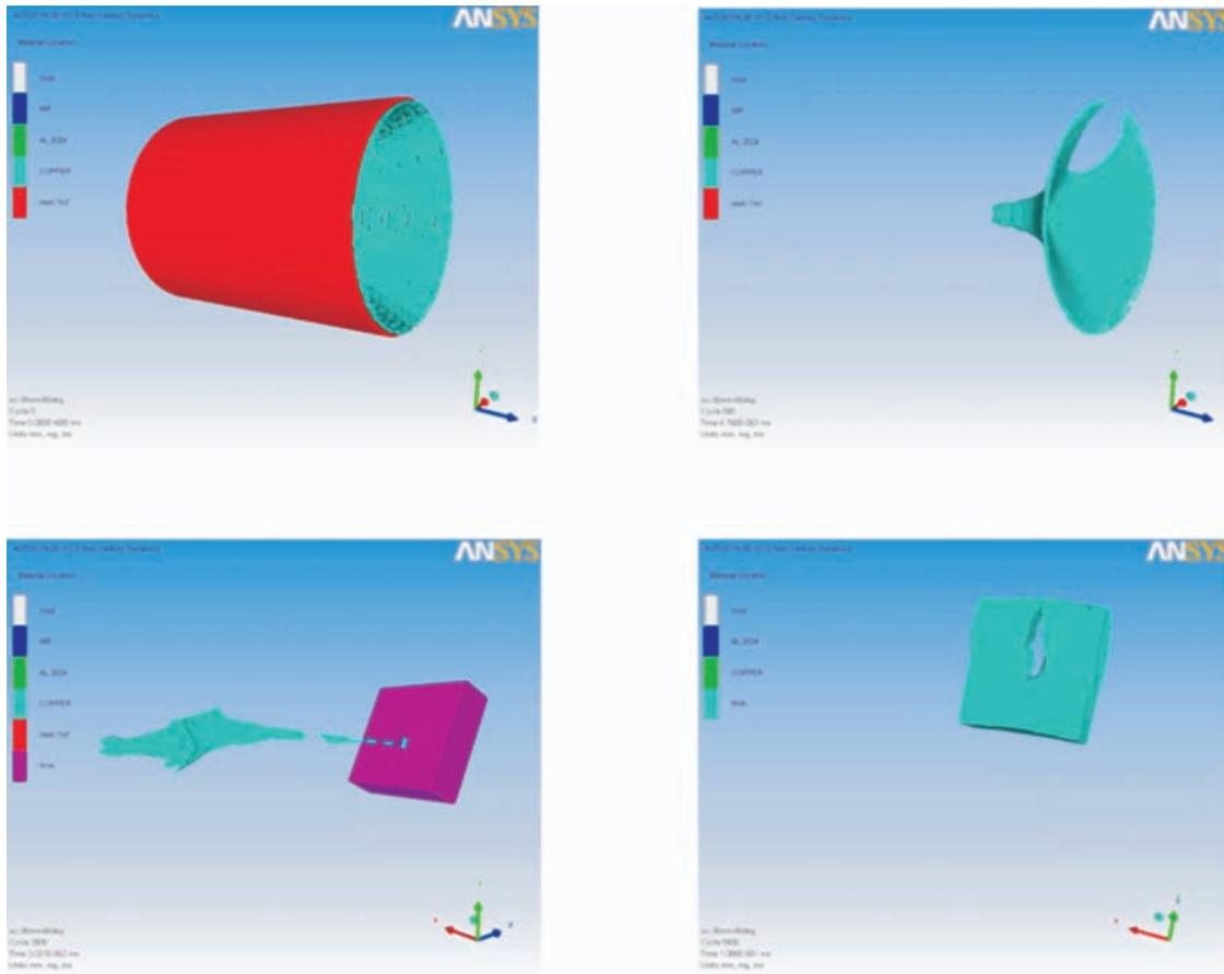
Figure 7. Simulation showing asymmetric collapse of MC liner resulting in an elongated crater on target.
