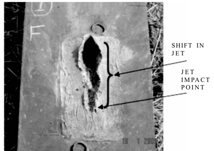
Figure 3. Penetration crater geometry.
