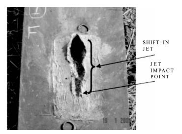
Figure 3. Penetration crater geometry.
