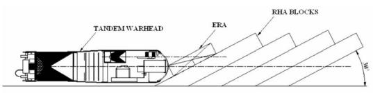
Figure 2. Warhead test set up.
