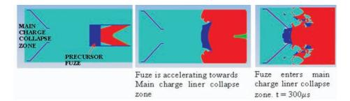
Figure 6. Hydrocode simulation of precursor blast.
