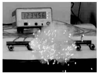
Figure 8. Multi point laser ignition.
