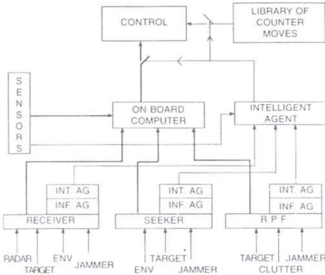
Figure 4. Interconnection of sub-systems in a missile with multiple intelligent agents.
