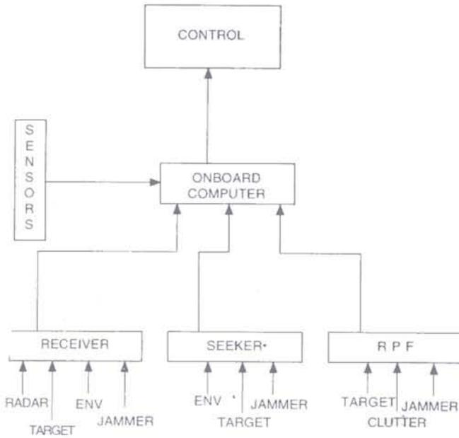
Figure 1. Conventional interconnection of sub-systems in a missile.
