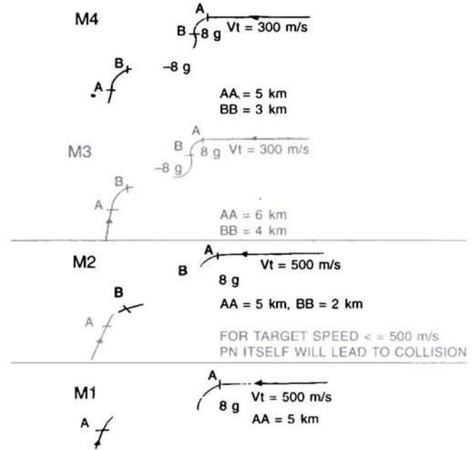
Figure 2. Typical missile-target maneuvers
