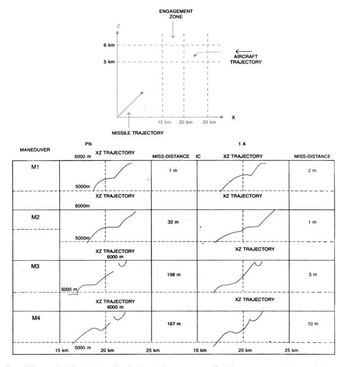
Figure 3. Target and missile trajectories with and without intelligent agent control for different maneouvers in the terminal phase in engagement zone.
