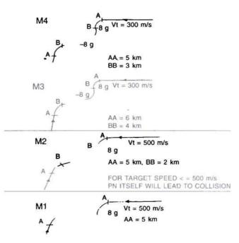
Figure 2. Typical missile-target maneouvers
