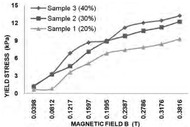
Figure 10. Yield stress function of per cent by volume as suspensions and magnetic field.
