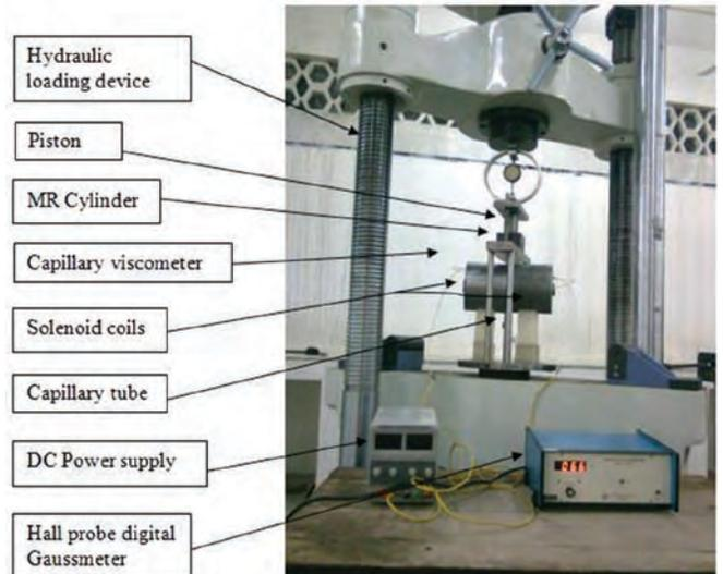
Figure 6. Photograph of test set-up to determine rheological properties of MR fluid.
