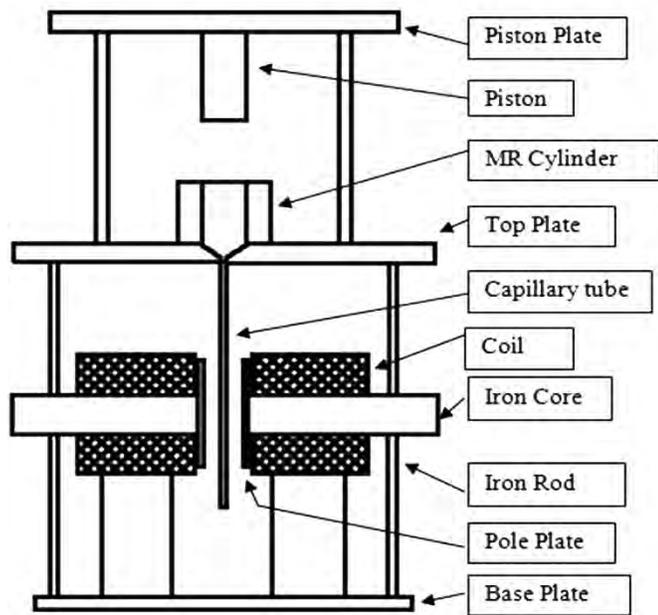
Figure 5. Capillary viscometer.
