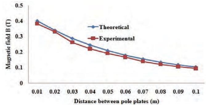
Figure 3. Comparison of theoretical and experimental magnetic fields at gap of 0.01 m.
