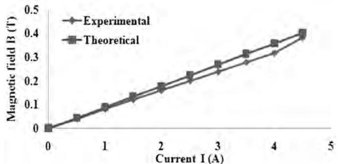
Figure 4. Comparison of theoretical and experimental magnetic fields at different currents for OA to 4.5 A..
