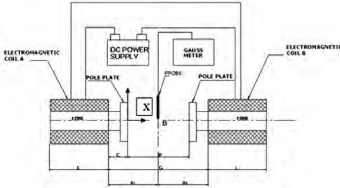
Figure 2. Electromagnetic circuit.
