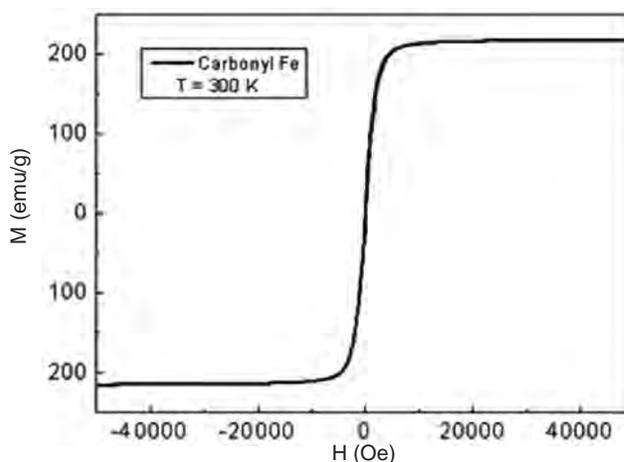
**Figure 1. Hysteresis curve for carbonyl iron powder.**
