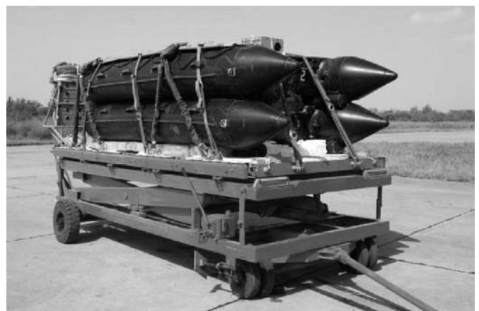
Figure 15. Duck drop system for AN-32.
