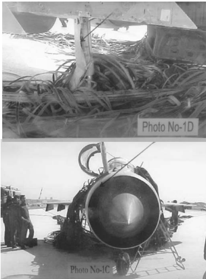
Figure 18. Successful engagement of aircraft in AABS at Sirsa, AF Station.
