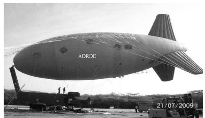
Figure 28. 2000 cum aerostat developed by ADRDE.
