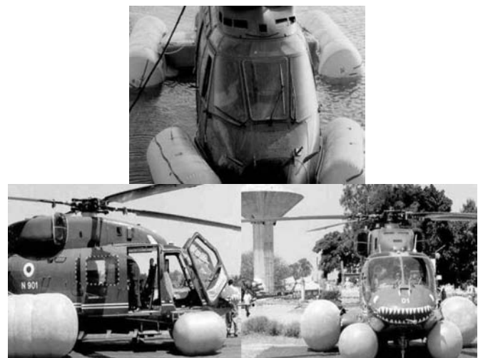
Figure 20. Floatation systems developed.
