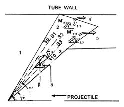
Figure 2. Flow over the projectile cone
