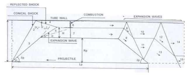
Figure Flow processes in detonation type ram accelerator
