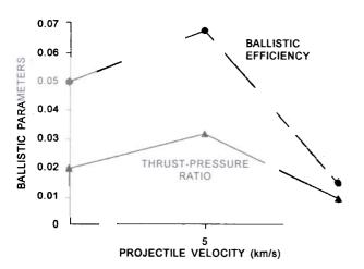
Figure 3. Variation of ballistic parameters with projectile velocity.
