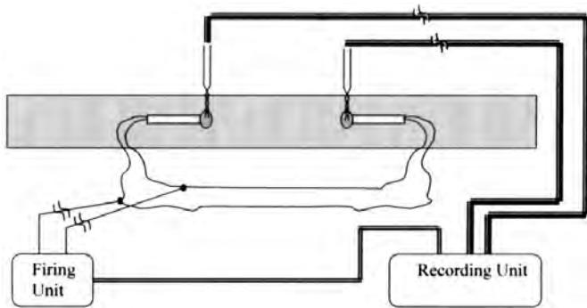
**Figure 1. Schematic of the field set-up used for the delay time and jitter measurements of electrical detonator no. 33.**
