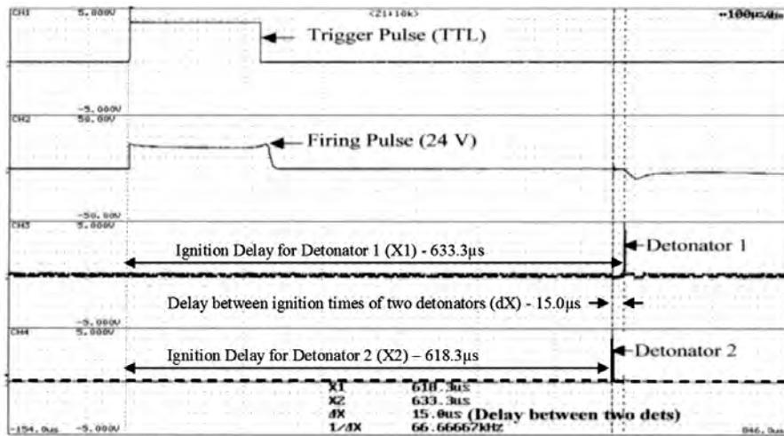
Figure 3. Recorded data signal for delay in ignition time and jitter for electrical detonator no. 33.
