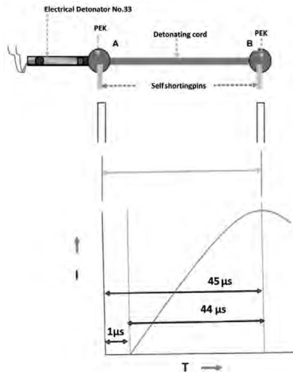
Figure 4. Schematic of charge assembly for optimisation of detonating cord length to synchronise the event of explosion of explosive at peak current in solenoid.
