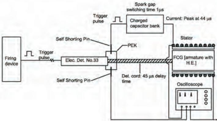
**Figure 5.** Block diagram for the timing circuit of seed current in stator, high explosive in armature and triggering of the diagnostics.
