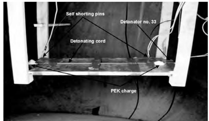
**Figure 2. Experimental set-up for the measurements in delay time precision.**
