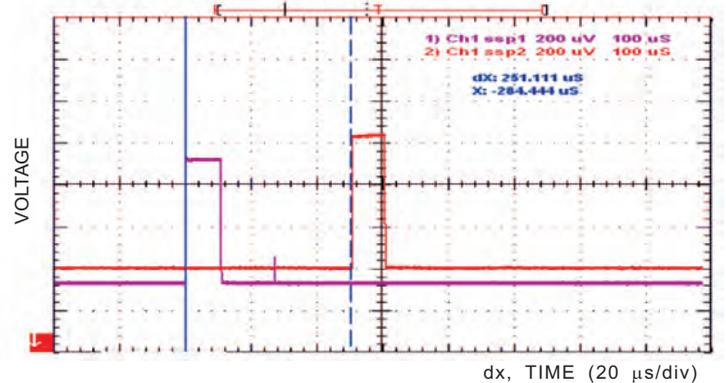
**Figure 6.** Measured delay time with waveforms for different prima cord lengths (*l*) and observed delay time (*dx*), as recorded on fast storage oscilloscope: (a) *l*=230 mm, *dx*=31.3 μs, (b) *l*=330 mm, *dx*=41.5 μs, and (c) *l*=1840 mm, *dx*=251.1 μs
