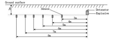
Figure 5. The experimental setup sketch.
