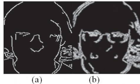
**Figure 2. Canny edge detector output on (a) un-normalized image (b) normalized image.**
