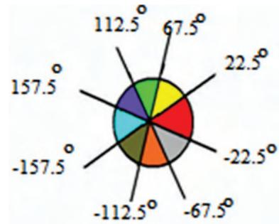
Figure 4. Quantization of gradient direction into eight bins.
