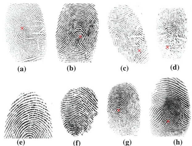
Figure 6. FVC2002 (a) and (b) correct corepoint detection; (c) and (d) failure cases; (e) and (f) missing core points; (g) and (h) tented arch images.
