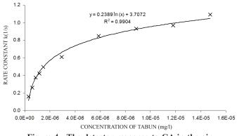
Figure 4. The detector response to GA in the air.
