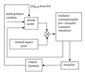
Figure 3. Block diagram of guidance algorithm.
