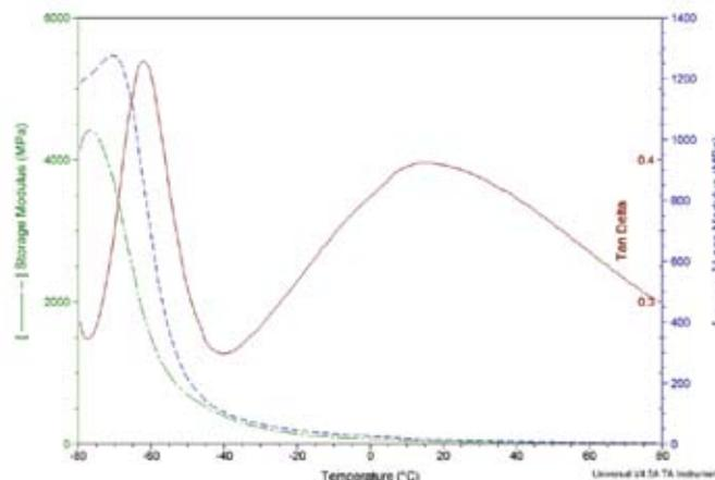
**Figure 1. DMA result for a standard sample at 11 Hz with 0.01 per cent oscillatory strain at heating rate of 2 °C.**
