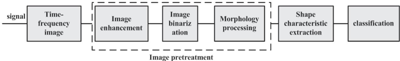
Figure 1. The process of proposed radar signal recognition method based on time-frequency image.
