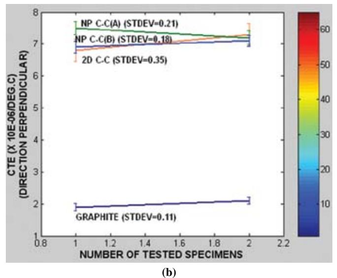
Figure 5. CTE of investigated specimens in direction (a) parallel (b) perpendicular.
