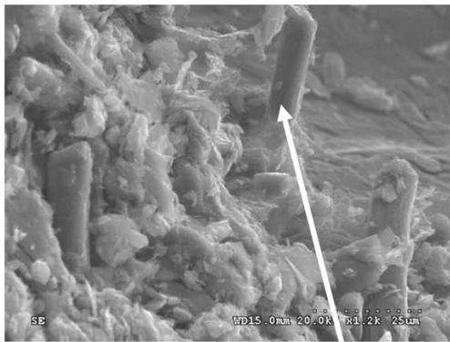
(e) Protrusion of sheared fibers
