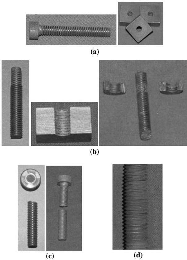
Figure 4. (a) C-C bolt and nut (size M6), (b) Thread shear failure in screw, nut and bolt, (c) Bolt failure, and (d) Stud post test (under 400N load at 1500 °C for 300 h).
