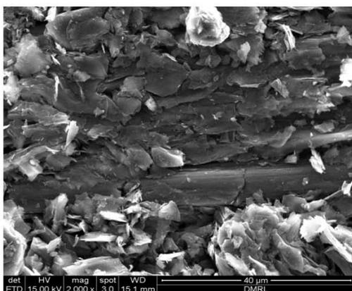
(i) Matrix crack in 2D C-C
