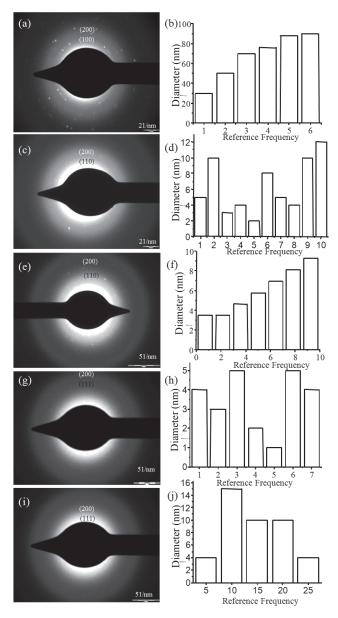
Figure 6. SAED and size distribution profiles of (a) and (b)  $LaFeO_3$ , A site doped  $La_{I-x}Ag_xFeO_3$  (c) and (d) x = 0.25, (e) and (f) x = 0.75, and B site doped  $LaFe_{(I-x)}Ag_xO_3$  (g) and (h) x = 0.25 and (i) and (j) x = 0.75.
