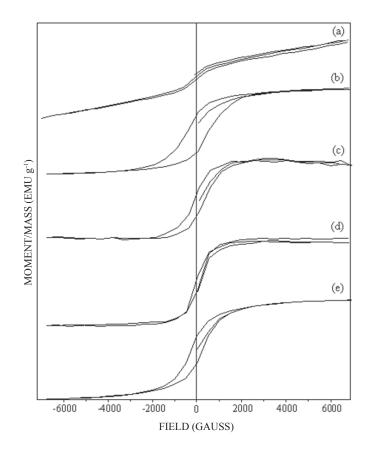
Figure 8. Magnetograms of (a)  $LaFeO_3$ , (b)  $La_{0.75}Ag_{0.25}FeO_3$ (c)  $La_{0.25}Ag_{0.75}FeO_3$ , (d)  $LaFe_{0.75}Ag_{0.25}O_3$ , and (e)  $LaFe_{0.25}Ag_{0.75}O_3$ .
