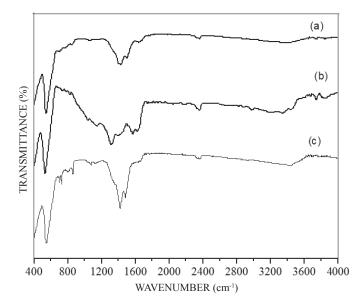
Figure 1. FT-IR spectra of samples (a)  $LaFeO_3$ , (b)  $La_{0.75}Ag_{0.25}FeO_3$ , (c)  $LaFe_{0.75}Ag_{0.25}O_3$ .
