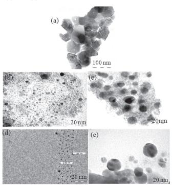
Figure 5. Transmission electron micrographs of (a) LaFeO<sub>3</sub>, (b) and (c) A site doped  $La_{(1-x)}Ag_xFeO_3$  (x = 0.25 and 0.75) and (d) and (e) B site doped  $LaFe_{1x}Ag_xO_3$ (x = 0.25 and 0.75).
