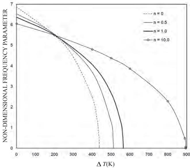
**Figure 6. Effect of material distribution on fundamental frequency of FGM beam in uniform temperature field ( $L/h = 10$ , C-C, TD).**
