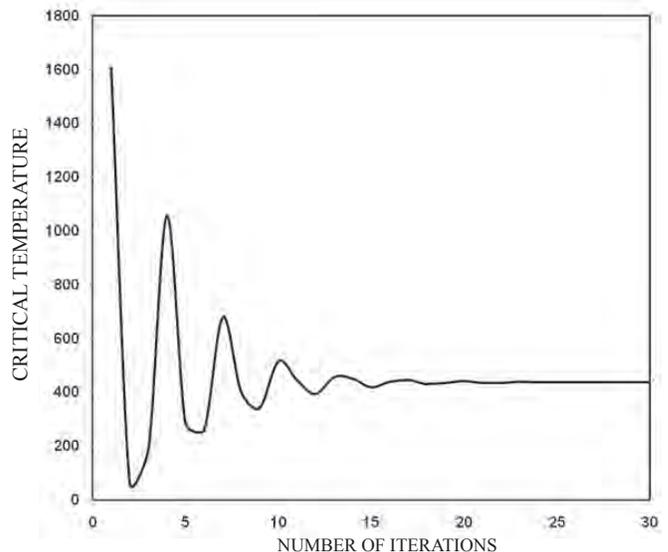
**Figure 4. Critical temperature vs Number of iterations (L/h = 10, n = 0, C-C).**
