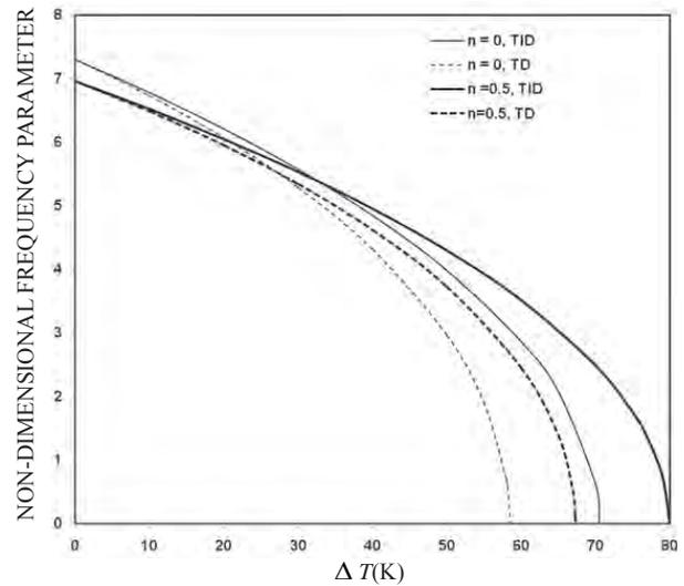
**Figure 5. Effect of temperature dependent material properties on fundamental frequency ( $L/h = 50$ , C-C).**
