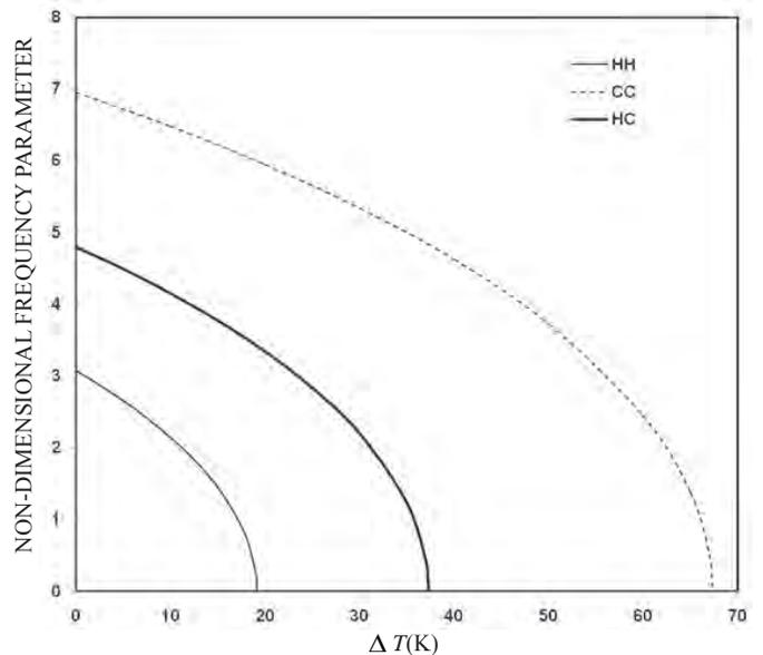
**Figure 8. Effect of boundary conditions on fundamental frequency of FGM beam in uniform temperature field ( $L/h = 50$ ,  $n = 0.5$ , TD).**
