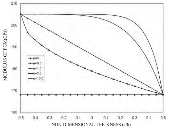
**Figure 2. A typical variation of Young’s modulus of FGM through thickness (at 300 K).**
