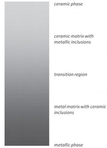
**Figure 1. A typical cross section of FGM beam with ceramic and metal as constituent materials.**
