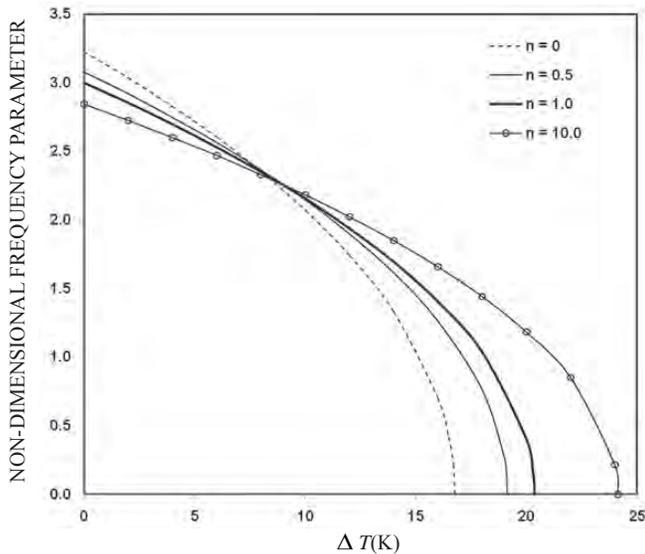
**Figure 7. Effect of material distribution on fundamental frequency of FGM beam in uniform temperature field ( $L/h = 50$ , H-H, TD).**
