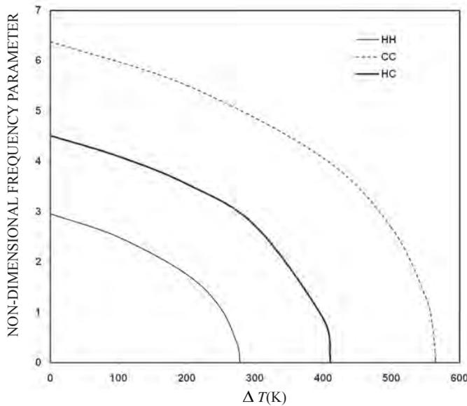
**Figure 9. Effect of boundary conditions on fundamental frequency of FGM beam in uniform temperature field (L/h = 10, n = 1.0, TD).**
