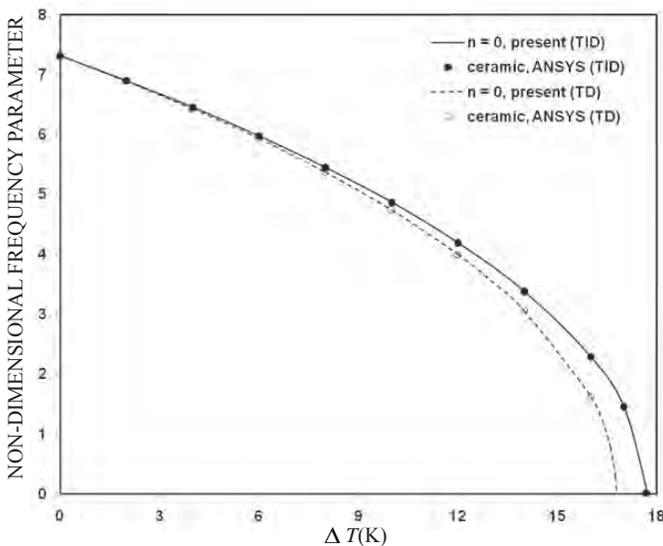
**Figure 3. Fundamental frequency vs FGM beam temperature (L / h = 100, n = 0, C-C).**
