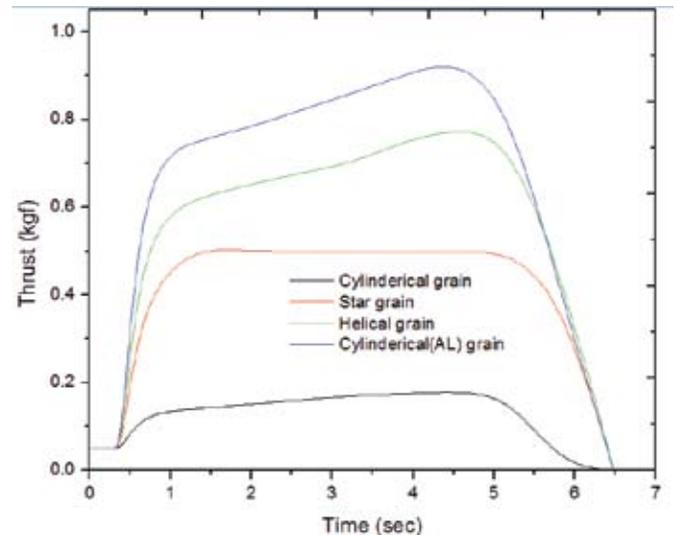
Figure 11. Thrust-time traces for 344.7 kPa.
