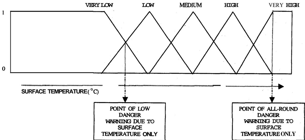
Figure 4. Fuzzification graph of snow surface temperature
