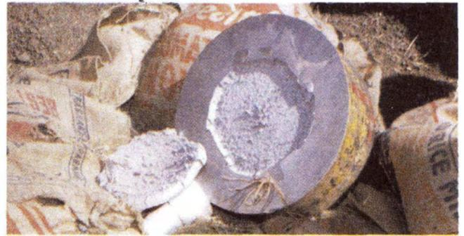
Figure 9. Scab from 100 mm diameter charge
