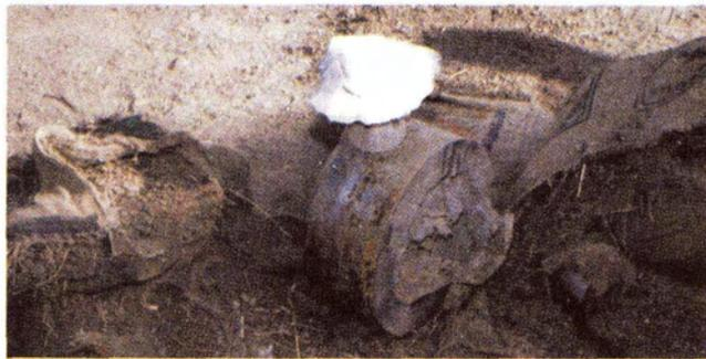
Figure 8. Scab from 150 mm diameter charge
