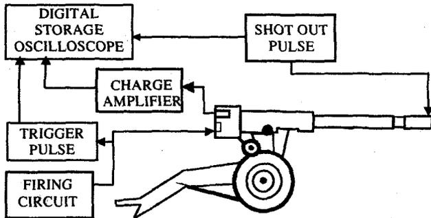
Figure 2. Schematic of breech pressure measurement setup.
