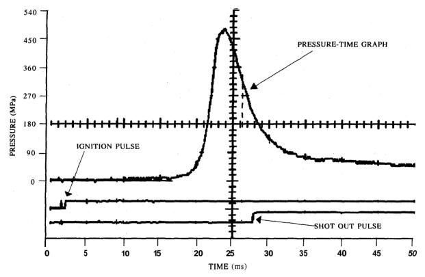
Figure 3. Typical record of breech pressure measurement
