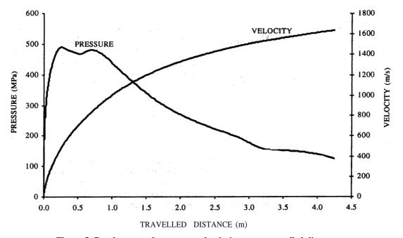
Figure 5. Development of pressure and velocity versus travelled distance
