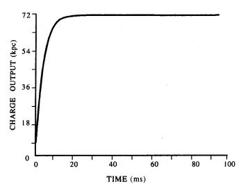
Figure 1. Charge output versus time graph of dynamic calibration of pressure transducer.
