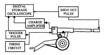
Figure 2. Schematic of breech pressure measurement setup.
