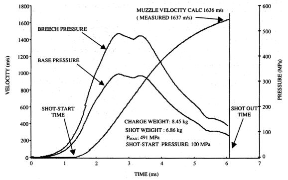
Figure 4. Development of velocity and pressure versus time
