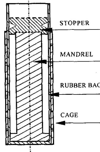
Figure 3. Wet bag isostatic pressing
