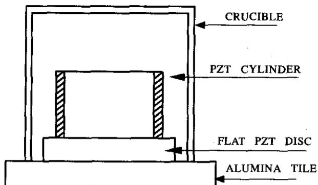
Figure 5. Sintering of PZT cylinder
