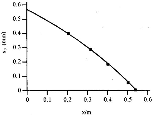
Figure 2. Plot of relative displacements of the fuel within the shell at different positions in projection acceleration process.
