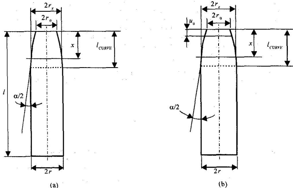
Figure 1. Displacement of fuel within shell in projection acceleration process: (a) before overloading and (b) after overloading
