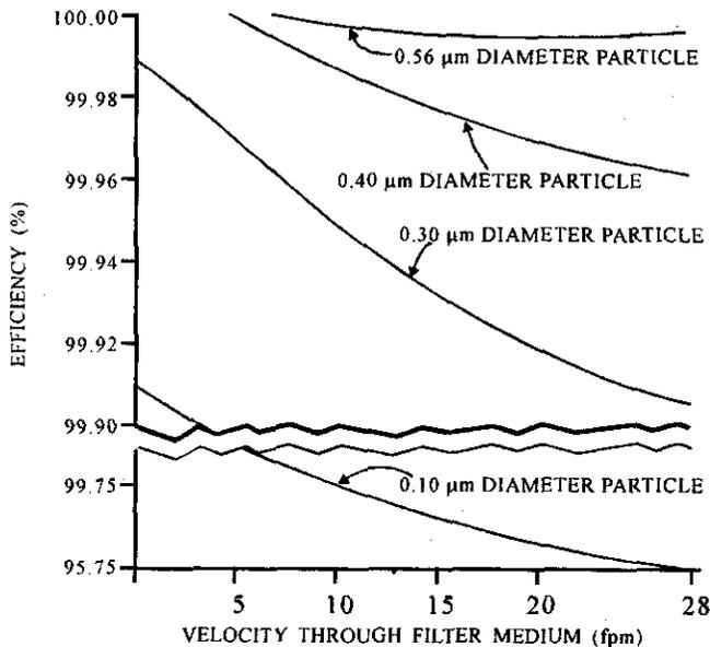
Figure 2. Penetration of HEPA filter medium by sub-micron particles as function of flow rate through medium.
