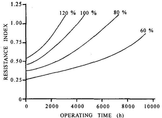
Figure 1. Effect of underrating on service life of extended medium filters, based on percentage of manufacturer's rated air flow capacity.
