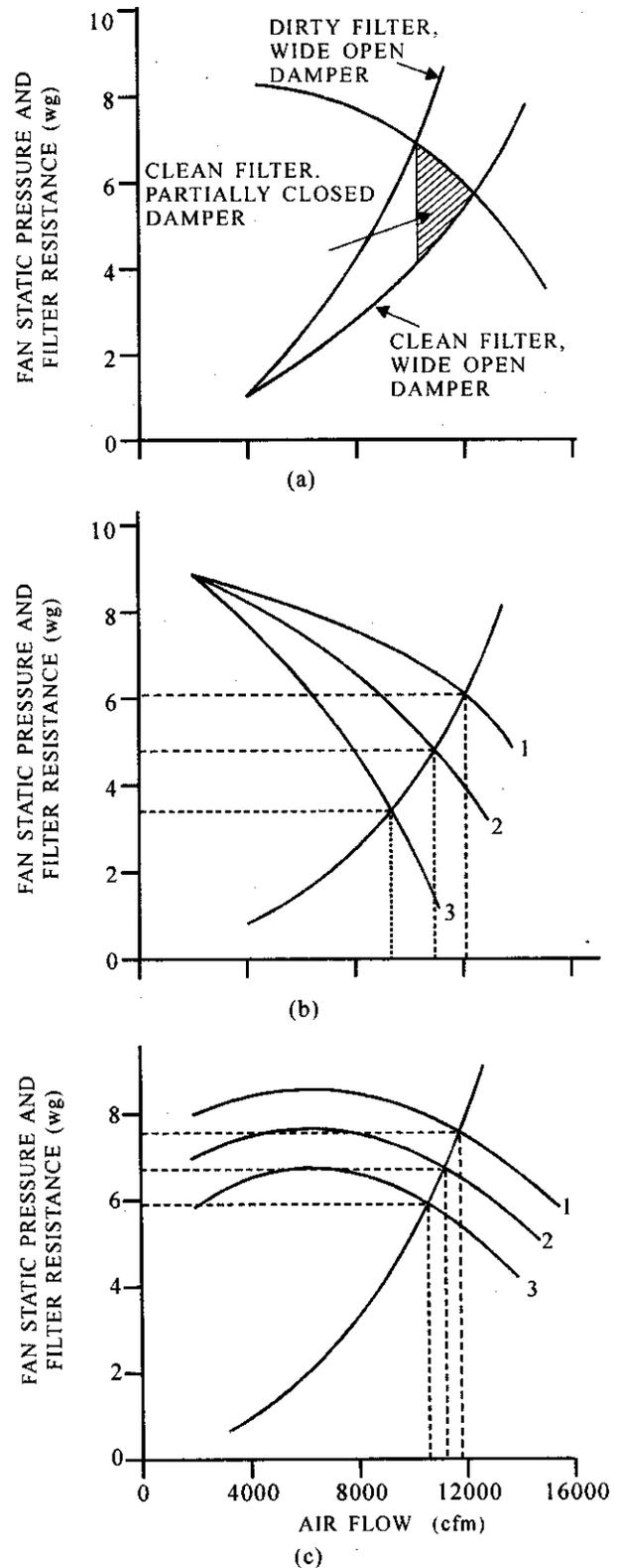
Figure 5. Comparison of fan and system operating characteristics with different methods of airflow control: (a) damper control (b) inlet vane control, and (c) variable speed control.
