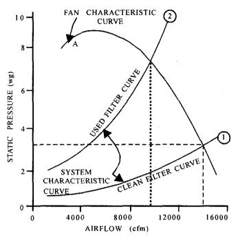
Figure 3. Fan and system characteristic curves showing relationships between airflow delivery and resistance.
