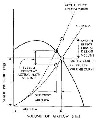
Figure 4. Result of selecting a fan on the basis of manufacturer's ratings. Curve A shows calculated duct system curve with no allowance for system effect.
